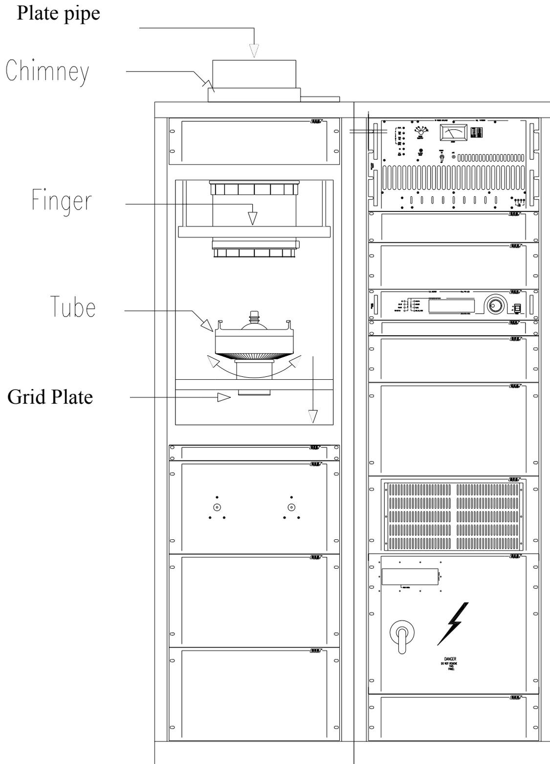
FIG. 14 TUBE INSTALLATION DIAGRAM N°3
