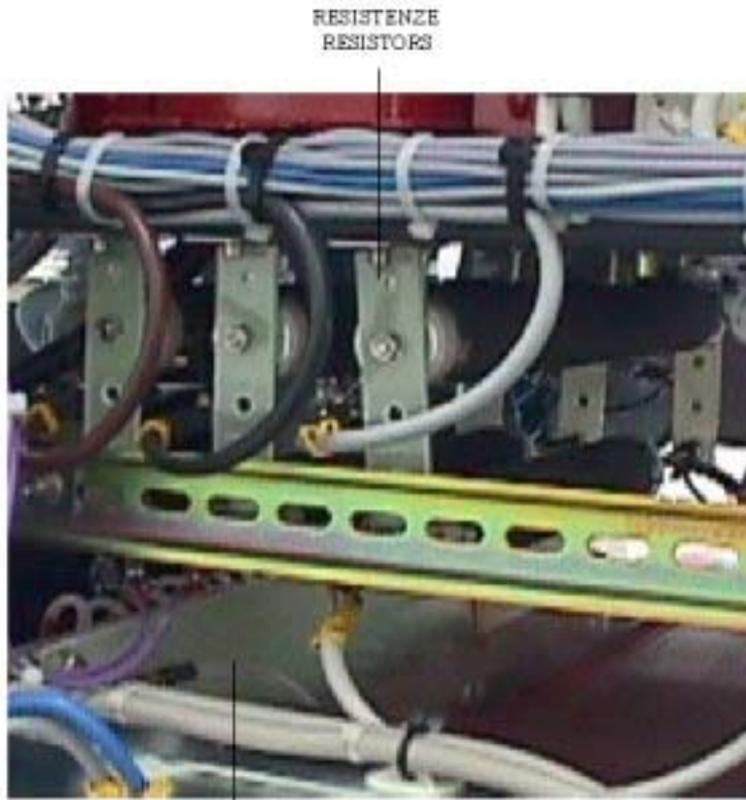
PONTE DI DIODI RADDRIZZATORE TENSIONE DI PLACCA
