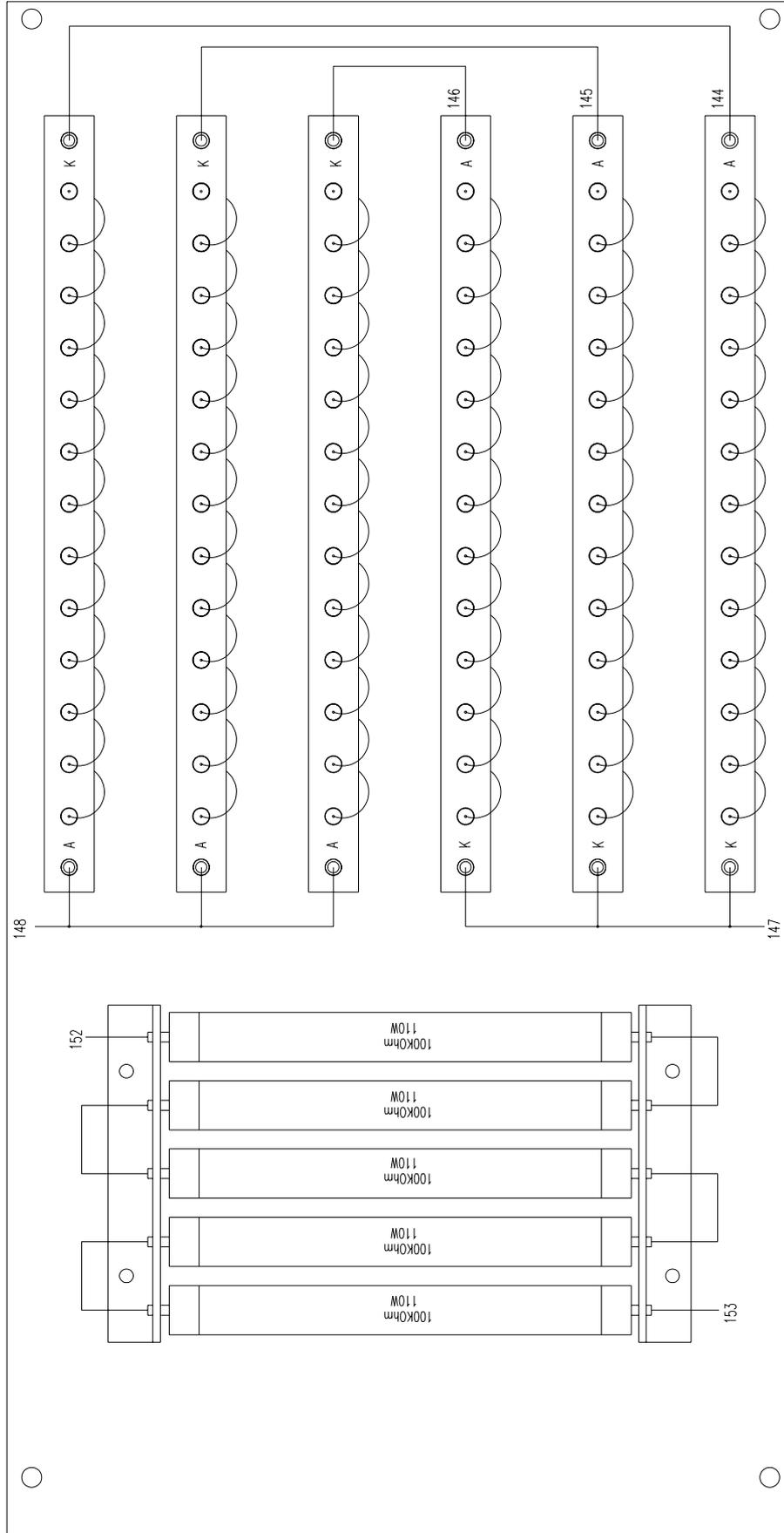
PONTE DI DIODI RADDRIZZATORE TENSIONE DI PLACCA
